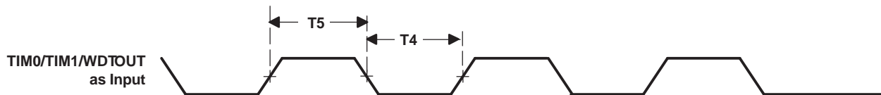
Figure 5-28. TIM0/TIM1/WDTOUT Timings When Configured as Timer Input Pins
